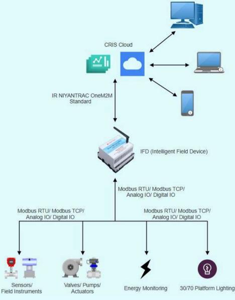
Working Principle of Wireless Device IFD
